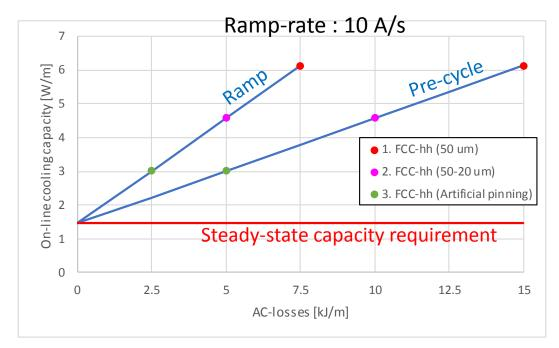
Capacity increase by a factor 2 to 4 w/r to steady-state requirement
