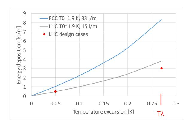
With the present helium inventory (33 l/m) and an initial temperature of 1.9 K, it is possible to buffer:
