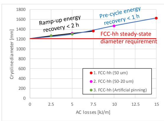
For Case 1 and 2 the cryoline is becoming larger than the magnet cryostats
