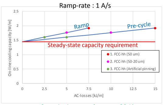
Capacity increase by up to 33 % w/r to steady-state requirement...
