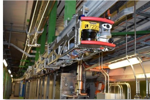
CERNbot for inspection and telemanipulation
