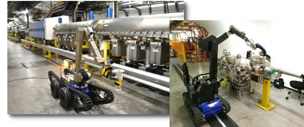
Telex and Teodor for inspection and telemanipulation
