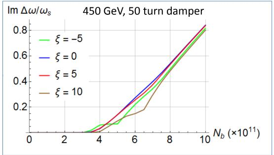
Destabilizing effect of the resistive damper See E. Métral, IPAC18, Vancouver, 04/2018
