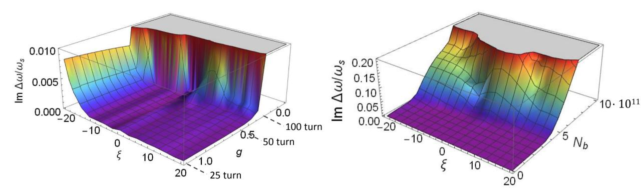
Damper gain: g = damping rate /  $\omega_s$
