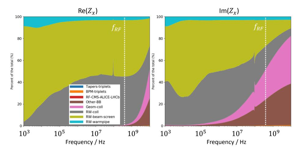
• Collimators and beam screen are the main contributors to the impedance
