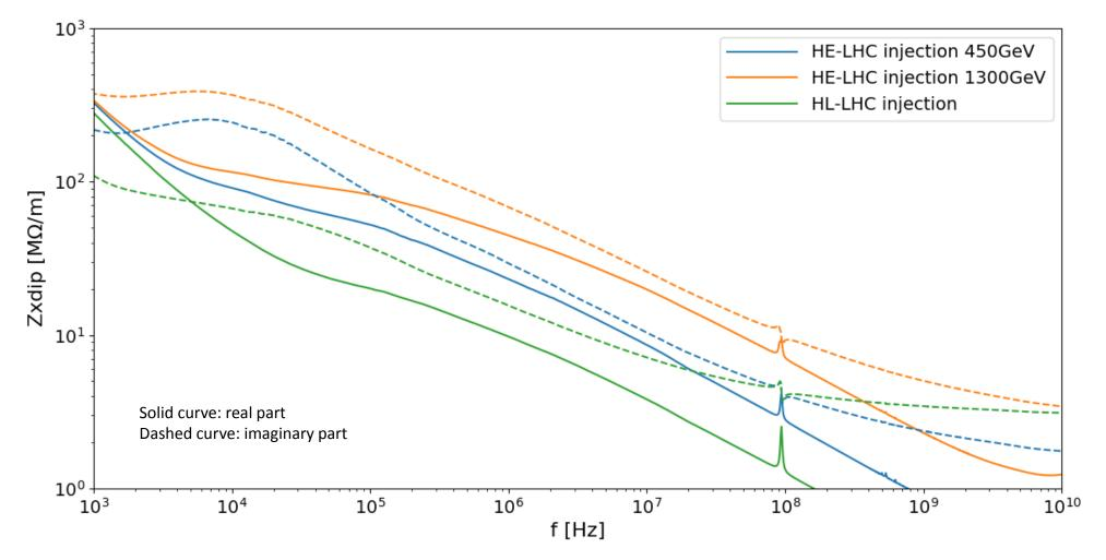
• 1.3TeV scenario has a larger impedance, because of the tighter collimator gaps
