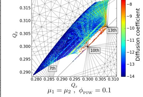
A nonzero crossing angle destroys the symmetry, the improvement is negligible compared to the case with zero crossing angle.
