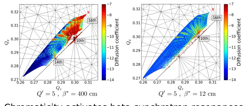
Chromaticity activates beta-synchrotron resonances. The effects of the hourglass effect and chromaticity seem to cancel, leaving an optimal  $\beta^*\approx 12$  cm. This is not affected significantly by a crossing angle.
