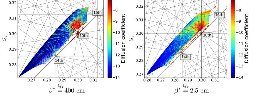
The hourglass effect causes mixing of the longitudinal and transverse dof, and activates beta-synchrotron resonances. The odd resonances are not affected.
