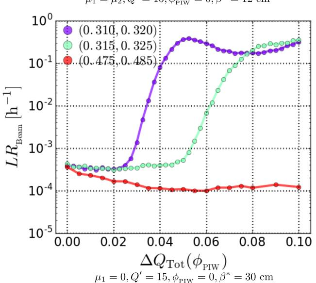
Setting  $\mu_1$ =0 and using the FCC design  $\beta^*$ , drastically reduces the maximal  $\Delta Q_{\text{Tot}}$ . From the LHC tunes, the limit is approximately 0.035. This is with zero asymmetrical effects in the beambeam interaction, and thus no odd resonances.
