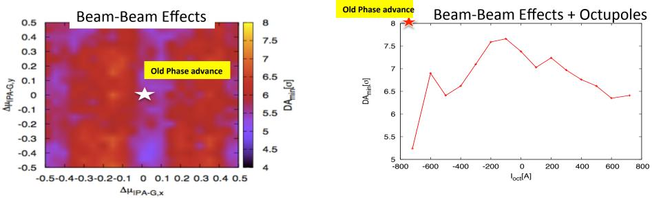
Strong dependency on IPs phase advance observed with beam-beam
