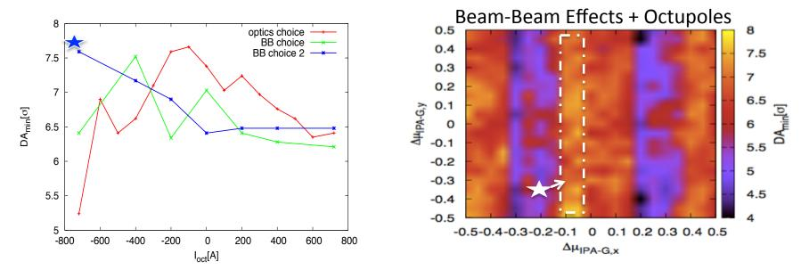
Further optimization of phase advance with beam-beam and octupoles compensation  $\rightarrow$  Will further change with multipolar errors
