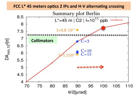
**Dynamic Aperture** from beam-beam effects larger than collimation aperture to do not increase the particle impact on collimation system due to BB diffusive mechanisms
