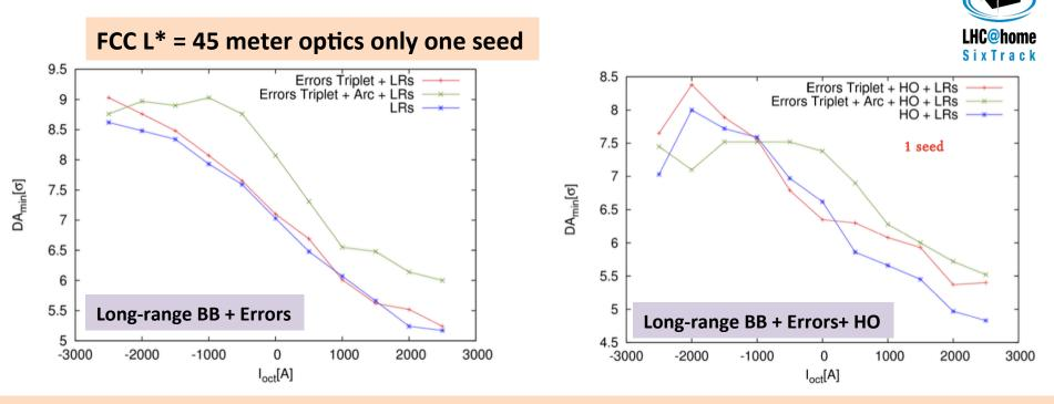
Break of long-range global compensation scheme in collision  $\rightarrow$  need further studies and lattice optimization L\* 40 meter optics under study with full seed statistics
