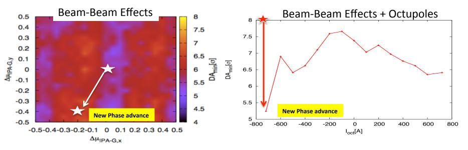
New Phase advance better for optics and beam-beam effects alone but breaks global compensation with octupole magnets (J. Barranco from Eurocircl 2017)
