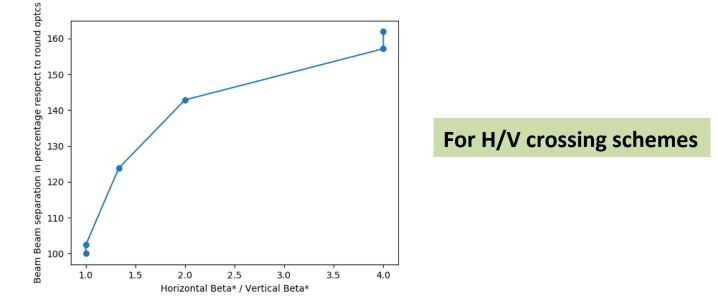
The extra separation needed from dynamic aperture studies with a DA goal of 6  $\sigma$  shows strong dependency on the beta\* ratio at the IPs
