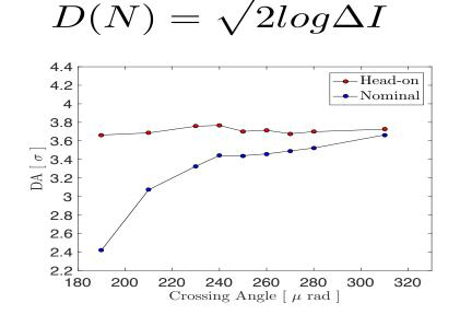
Head-on colliding bunch and nominal havesimilar losses at larger anglesFor separation below 8.3 σ long-range effectstake over@IPAC 2017 THPAB056
