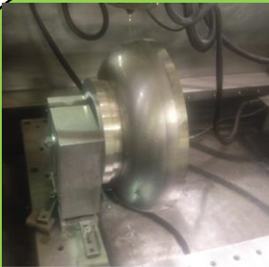
Half-cell during pre-trimming by wire electro-discharge machining and final milling for iris weld joint preparation
