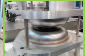
802 MHz RF measurement fixture for dumbbells and end-groups
