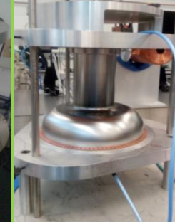
802 MHz RF measurement fixture for dumbbells and end-groups
