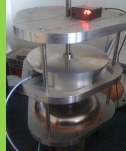
802 MHz RF measurement fixture for dumbbells and end-groups
