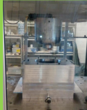
802 MHz half-cell deep-drawing and beam tube rolling dies
