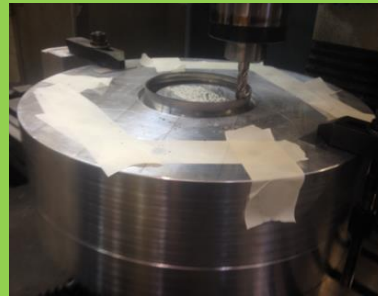
Half-cell during pre-trimming by wire electro-discharge machining and final milling for iris weld joint preparation
