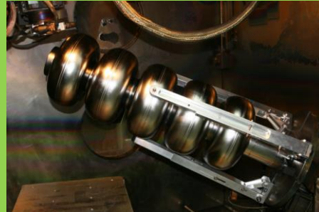
Five-cell cavity at various equator weld stages of sub-assemblies
