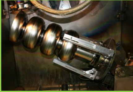
Five-cell cavity at various equator weld stages of sub-assemblies
