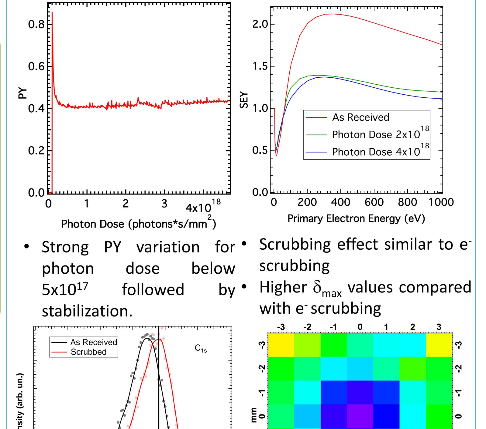
from a bending magnet in DA $\Phi$ NE , we performed the first test experiments following simultaneously gas desorption, PY, SEY and surface chemistry modification (by using XPS spectroscopy) during the focused WL irradiation of a LHC Cu sample at room temperature. The Photon Flux delivered to the sample is calculated by taking into account the total Photon Flux of DA $\Phi$ NE [4] and the reflectivity of all optical elements.
