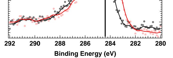
Modification of C 1s photoemission peak from surface impurities to graphitic carbon [3]
