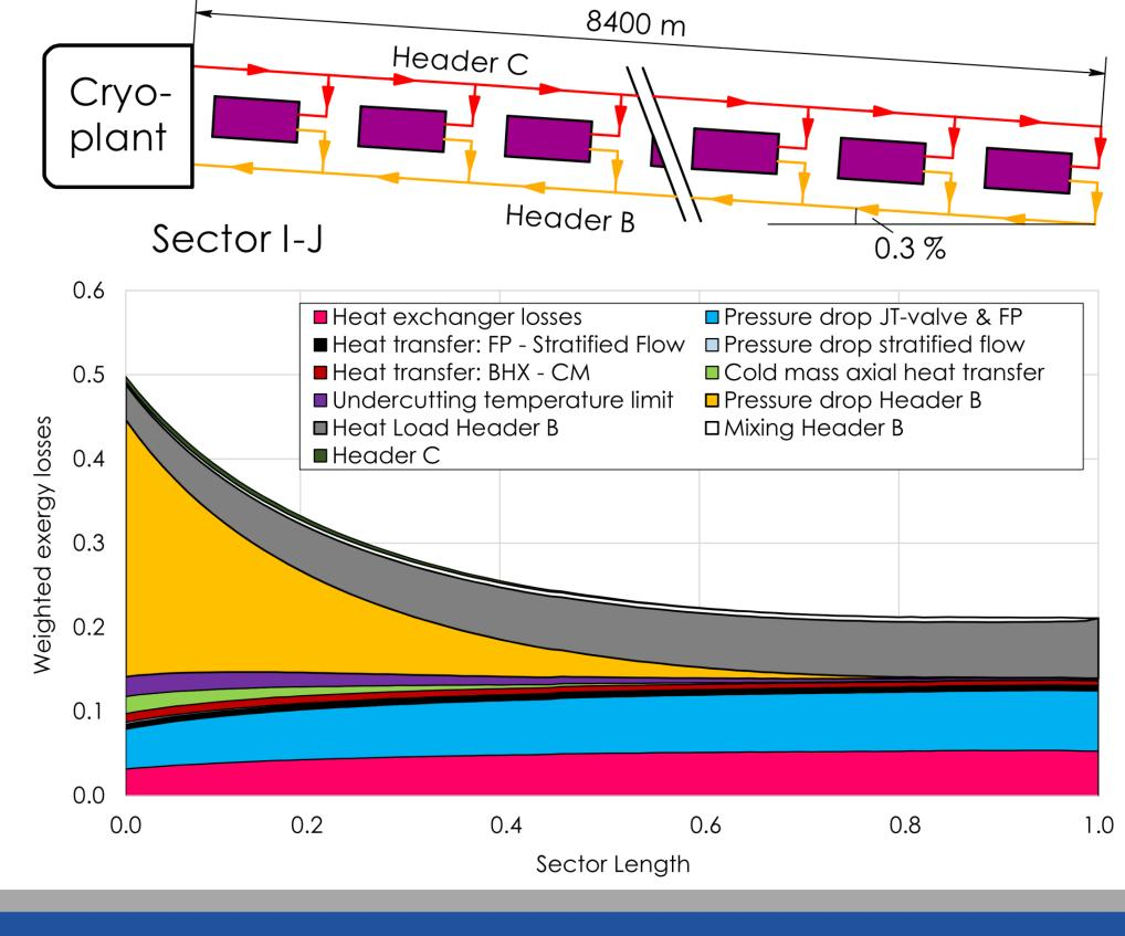
The arc of one long sector consists of 79 half-cells in series. Due to the slope of 0.3 % of the tunnel, the sector I-J cryoplant is about 30 m higher elevated than the last half-cell. Any low pressure helium vapour generated at the sector end has overcome hydrostatic pressure in addition to the frictional pressure drop. choking pumping line (header B), the determines requirements reach to cryoplant suction pressure.
