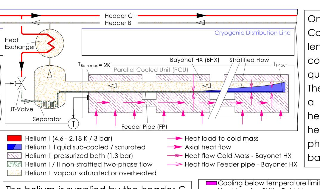
One parallel cooled Cold Mass Cooling unit corresponds to the length of an optical half-cell consisting of six dipoles and one quadrupol in series (≈107 m). The cold mass is immersed into a static bath of superfluid helium at 2 K (=  $T_{Bath\ max}$ ). The heat load is extracted by a twophase helium flow via the bayonet heat exchanger (BHX).
