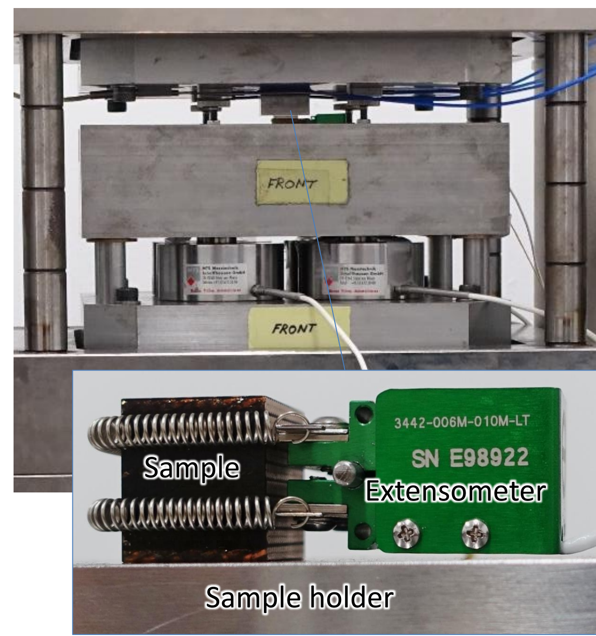
Fig. 3: Ten-stack sample with clip-on extensometer with 6 mm gauge length.
