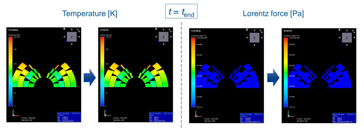
Temperature differences are increasing while Lorentz force is decreasing during discharge → Non trivial prediction of the moment of peak mechanical stress
