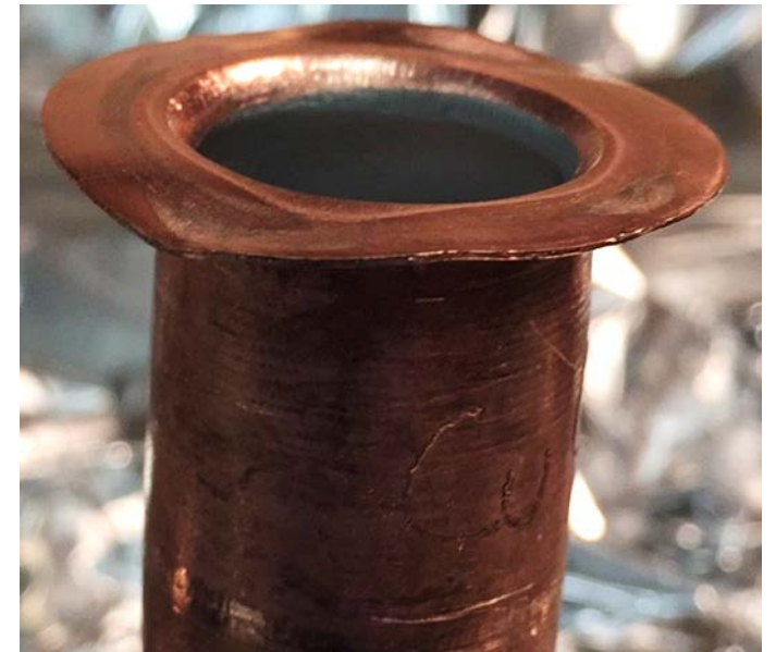
Bending of the flange at 650 °C
