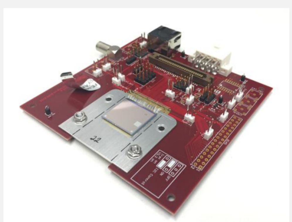
Single chip card with wire-bonded assembly
