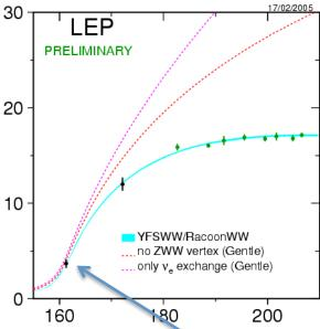
At LEP2  $Vs=161 \text{ GeV } \sigma=4pb$   $\epsilon=0.75, \ \sigma_B=300 \text{ fb}$   $p=0.9: \epsilon p\approx 0.68 \ (@161)$   $\Rightarrow m_W=80.40\pm 0.21 \text{ GeV}$ with  $11/pb \ @E_{CM}=161 \text{ GeV}$
