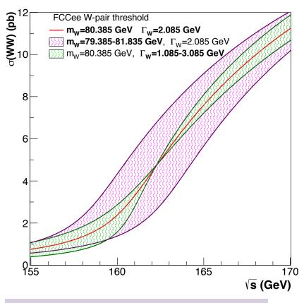
$d\sigma_{WW}/d\Gamma_{W} = 0$ at  $E_{CM}^{\sim}$ **162.3 GeV**  $^{\sim}$ 2m<sub>W</sub> + 1.5 GeV Measure oww in two energy points  $E_1$ ,  $E_2$  with a fraction f of lumi in  $E_1$
