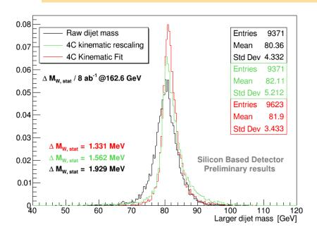
Smaller dijet mass tends to be off-shell Larger dijet mass is on-shell combined **statistical** uncertainties  $\Delta M_W$  (4C fit) = 1.02 MeV  $\Delta M_W$  (4C rescaling) = 1.18 MeV  $\Delta M_W$  (raw mass) = 1.55 MeV
