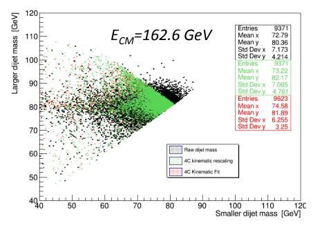
The expected statistical uncertainty on the W mass peak value ( $\Delta m_W$ , stat) is estimated with a **binned max likelihood fit** on the reconstructed  $m_W$  distributions, **using templates** with different nominal W mass values. The final expected uncertainty is the result of the combination of the measurements of the two reconstructed masses.
