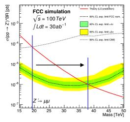
$Z' \rightarrow \mu\mu$  limit assuming FCC-hh vs. CMS detector performance (both at 100 TeV)
