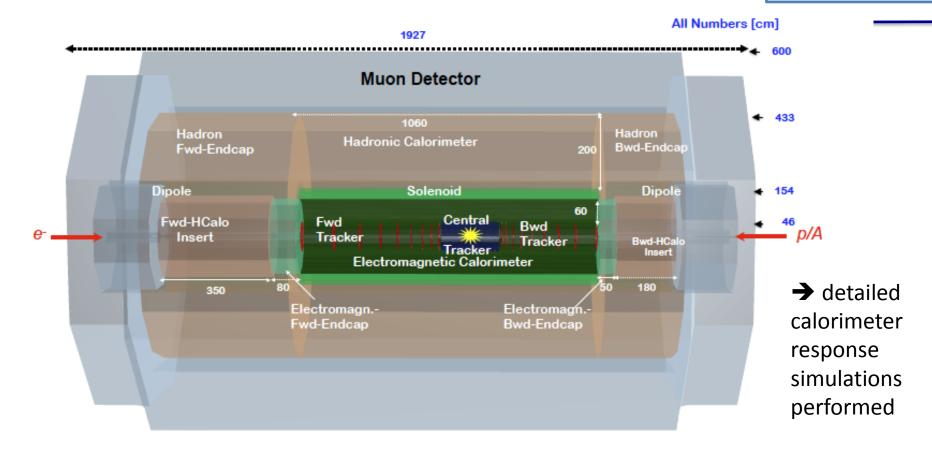
Based on the LHeC design; Solenoid&Dipoles between Electromagnetic Calorimeter and Hadronic Calorimeter. Length of Solenoid ~11m. detector setup in DD4hep.
