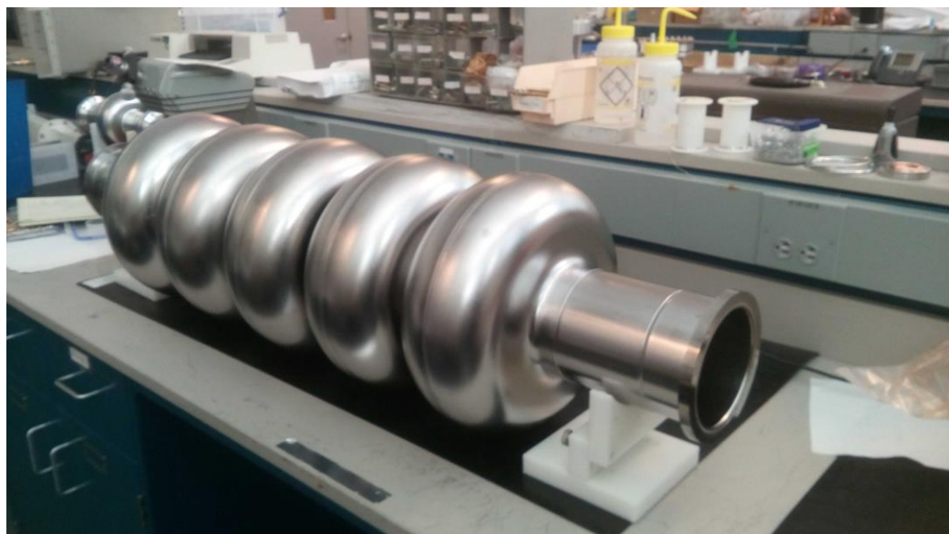
The first Nb 802 MHz 5-Cell cavity fabricated mid-October at JLAB
