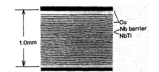
30 layers of NbTi, 8-10 micron thick, alternated with Cu for stabilization
