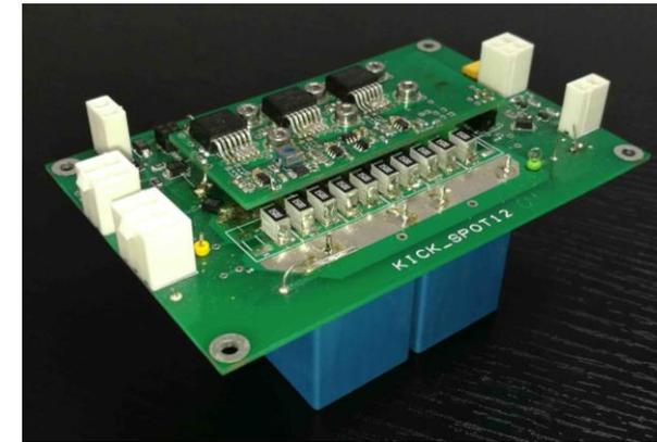
Switch unit: current sharing of 3 parallel MOSFETs:
