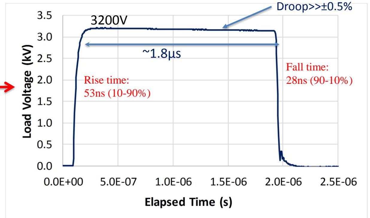
Circuit time constant of 24 ns with a load of 1.175  $\Omega \Rightarrow$  four stage Marx circuit inductance of  $\sim 28$  nH ( $\sim 7$  nH/stage).
