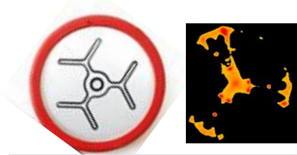
Illumination map above 12uJ threshold for 49uJ pulse
