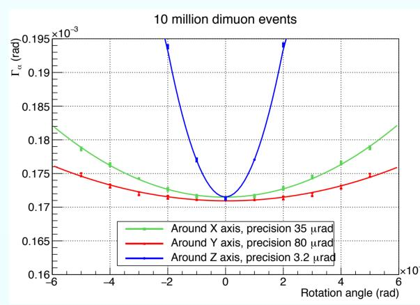
The precision on the Euler rotation angle around the y axis improves from 80 to 18  $\mu$ rad (in one hour at the Z pole) by also minimizing the correlation between  $\alpha$  and  $x_{\gamma}$ : such a rotation with respect to the natural frame mixes indeed the x ( $\alpha$ ) and z ( $x_{\gamma}$ ) information in a visible way:
