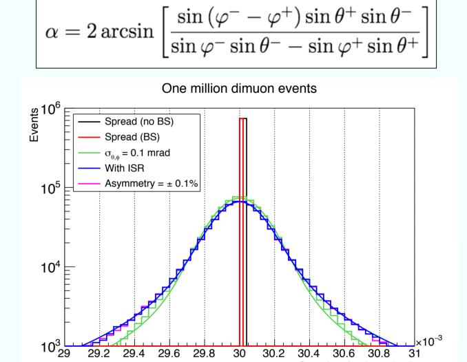
The spread of the  $\alpha$  distribution from dimuon events is smallest when the z axis (used to determine  $\theta^{\pm}$ ) and the x axis (used to determine  $\phi^{\pm}$ ) are perfectly known. The alignment of the detector with respect to these axes can therefore be achieved with a minimization of this spread. Precisions of 3.2 (35)  $\mu$ rad on the Euler rotation angles around the x (z) axes need only one hour at the Z pole.
