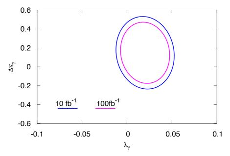
Two dimensional 95% C.L contour plot anomalous couplings in the  $\lambda_{\gamma}$  – $\Delta\kappa_{\gamma}$  plane for the integrated luminosity of 10 fb<sup>-1</sup> and 100 fb<sup>-1</sup> at FCC- ep with electron beam energy  $E_e$  =60 GeV with polarization P =–0.8 .
