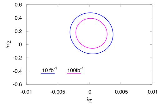
Two-dimensional 95% C.L contour plot of anomalous couplings in the  $\lambda_Z$  – $\Delta \kappa_Z$  plane for the integrated luminosity of 10 fb<sup>-1</sup> and 100 fb<sup>-1</sup> at FCC-ep with electron beam energy Ee=60 GeV with polarization P=-0.8.
