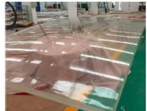
spherical sheet by thermal bending
