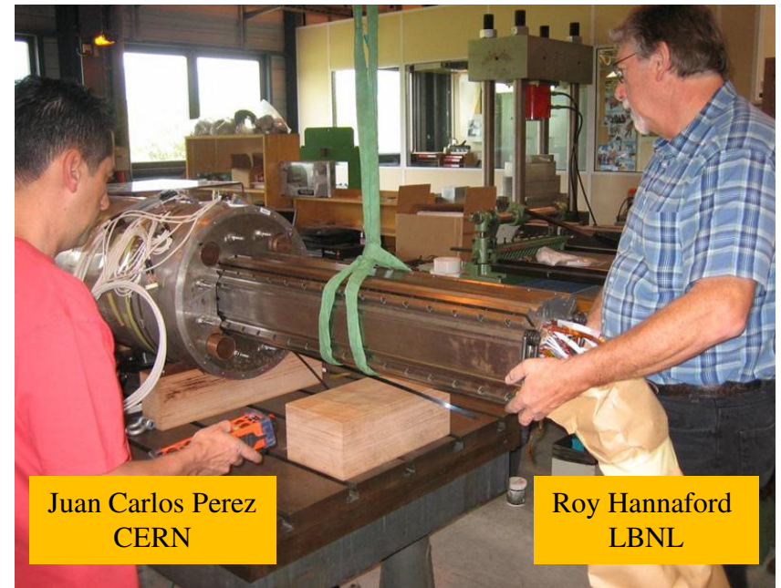
TQS assembly at CERN
