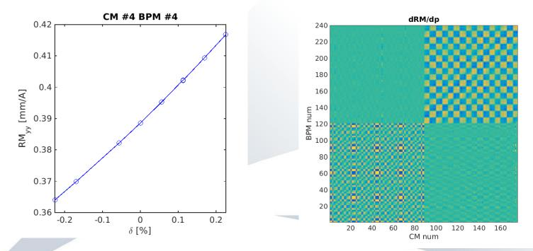
Both  $\partial ORM / \partial \delta$  and  $ORM^2$  depend linearly on the **sextupole** strengths and in principle can be used to fit the non-linear fields present in the machine.
