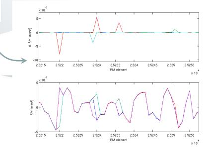
The phase in the coupled plane consistently gives values that do not follow the main plane oscillation. It is more pronounced for BPMs with the small signal amplitude:
