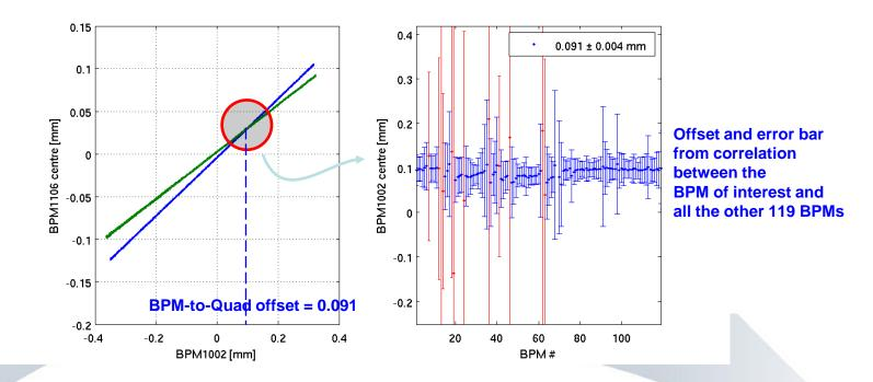
For BPM offset the Fast BBA gives 0.091±0.004 mm which agrees with usual DC BBA offset of 0.095±0.004 mm
