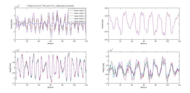
At 6Hz, the effect seems to be **4 times weaker**. Notice how the Pi/2 effect us unchanged by the skew magnet.
