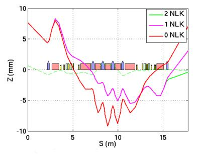
Orbits tracking in the first cell with the 2 MLKs
