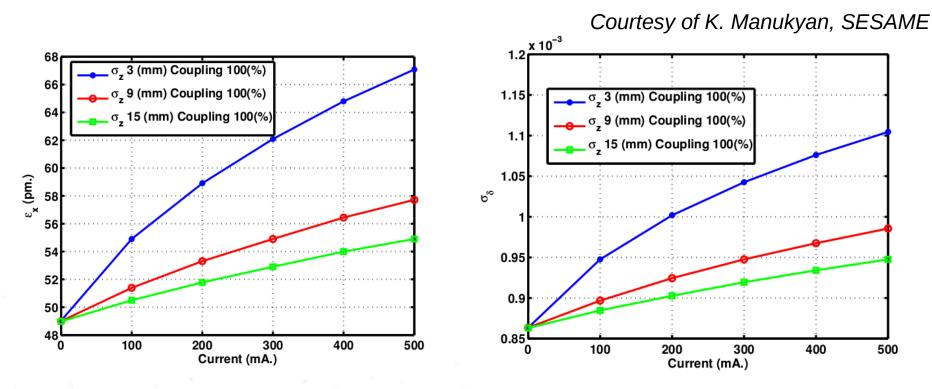
Preliminary IBS effect computed with Elegant code : Simple Gaussian distribution model ZAP code gives equivalent values
