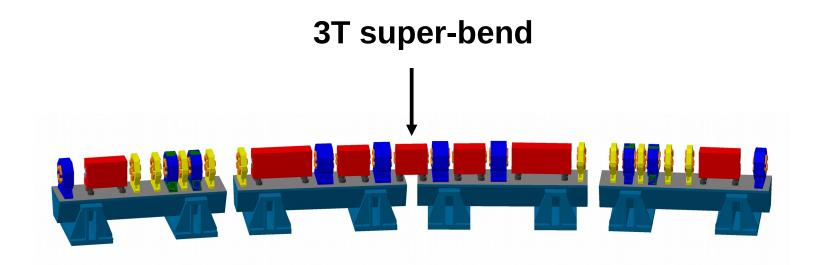
Insertion of 3T super-bend in the central magnet of the cell
