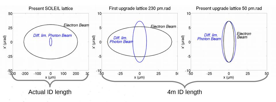
Diffraction limited photon beam emittance is 65 pm.rad at an energy of 3 keV
