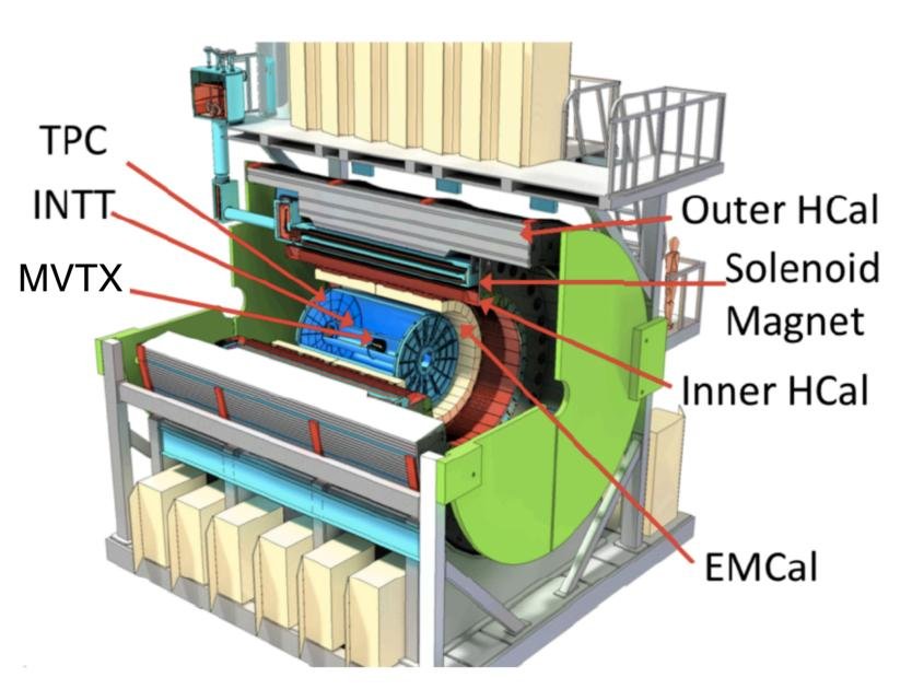
Uses BABAR superconducting solenoid (1.4 T) Recording rate for Au+Au collisions = 15 kHz
