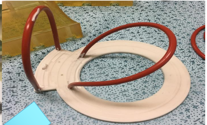
Vacuum / pressure Impregnation seal
