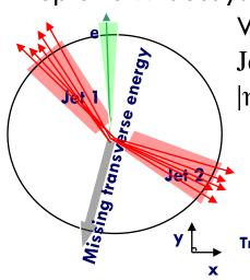
W $\rightarrow$ lv, where l=e or  $\mu$ Jet E<sub>T</sub>>20 GeV  $|\eta|<1.5$
