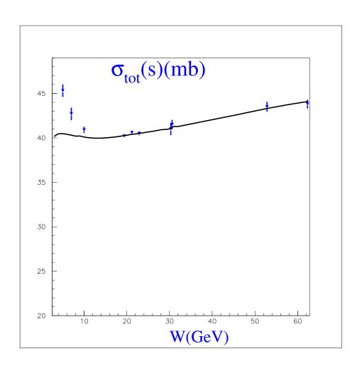
The total cross section  $(\sigma_{tot} = 1/2[\sigma_{tot}(pp) + \sigma_{tot}(p\bar{p})]).$  The curve illustrates our parametrization.
