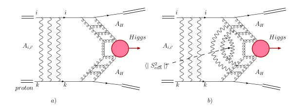
Fig-a shows the contribution to the survival probability in the G-W mechanism Fig-b illustrates the origin of the additional factor  $\langle \mid S_{enh}^2 \mid \rangle$
