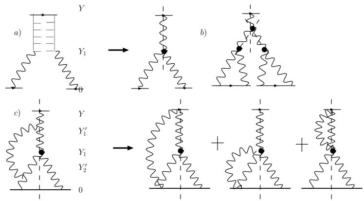
Examples of the Pomeron diagrams that lead to a different source of the diffractive dissociation that cannot be described in the framework of the G-W mechanism. (a) is the simplest diagram that describes the process of diffraction in the region of large mass  $Y - Y_1 = \ln(M^2/s_0)$ . (b) and (c) are examples of more complicated diagrams in the region of large mass. The dashed line shows the cut Pomeron, which describes the production of hadrons.
