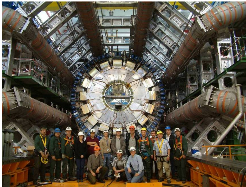
Calorimeter barrel after its move into the center of the detector (4 th November 2005)
