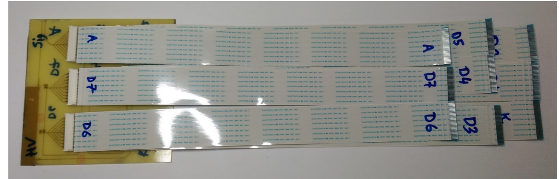
cables connecting SEE layers to HV divider
