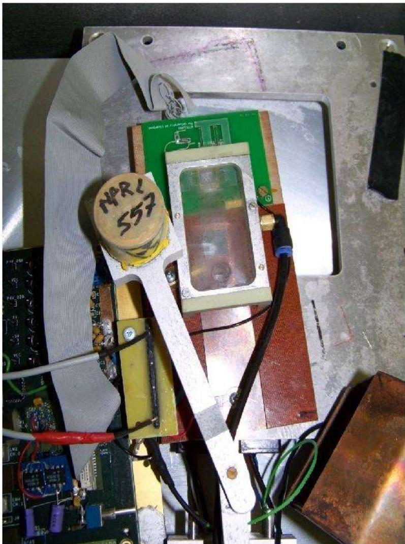
$^{90}\text{Sr}$  fast electron source used to generate signal.
