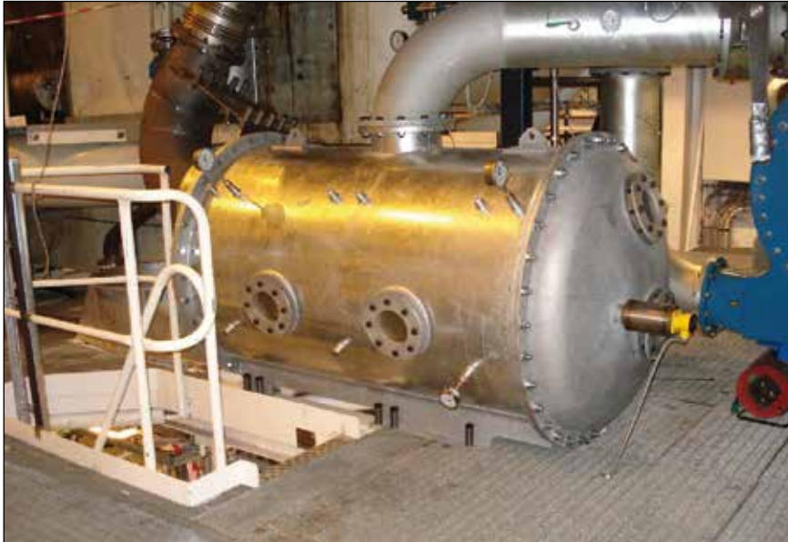
Fig. 17: The newly developed EGR scrubber applied to the test engine
