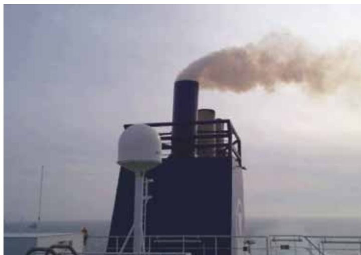
Figure 14: a vapour plume produced by an operating wet scrubber
