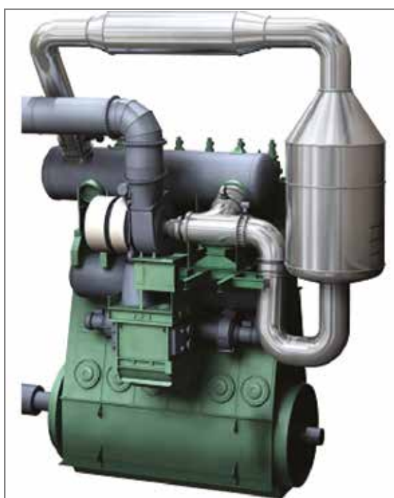
Figure 17: SCR arrangement – two-stroke low speed engine (image courtesy of MAN Diesel & Turbo)
