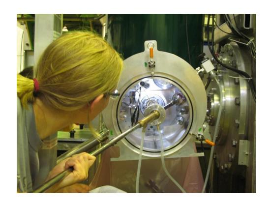
"side-loading" of samples into cryostat vacuum
