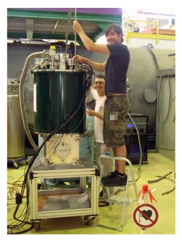
17 T, 60 mK to 300 K B'ham cryomagnet
