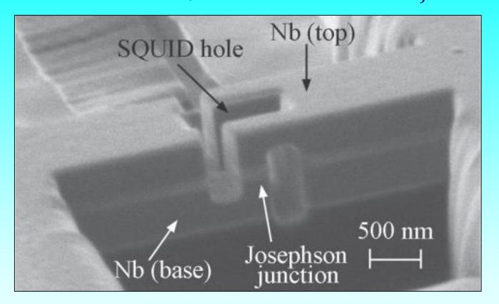
SEM images of a nanoSQUID fabricated by using the Focused Ion Beam (FIB) sculpting and the fully niobium technology. The flux capture area of the nanosensor is  $(1 \times 0.2)$  mm<sup>2</sup> and the two Josephson tunnel junctions have an area of about  $(0.3 \times 0.3)$  mm<sup>2</sup>.
