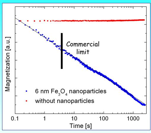
Magnetic relaxation measurement at T = 4.2 K of  $Fe_3O_4$  nanoparticles having an average diameter of 6 nm and cooled in a magnetic field of 10 mT (blue dots). The black straight line is an exponential fit of the data. The same measurement was previously performed without the nanoparticles (red squares).
