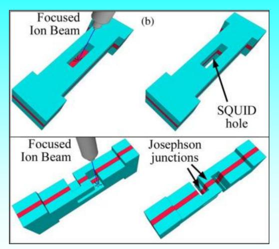
A rectangular hole is realized in the centre of the strip, resulting in two parallel lamellae and defining both the Josephson junction's width and the loop of the nanoSQUID device.
