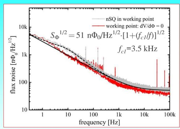
Flux noise spectral density measured at 4.2 K (gray line), and the corresponding fit is shown as a dashed black line. In magnetic insensitive working points, a behavior according to the red line has been observed, indicating critical current fluctuations as the main reason for the degraded low-frequency noise performance.
