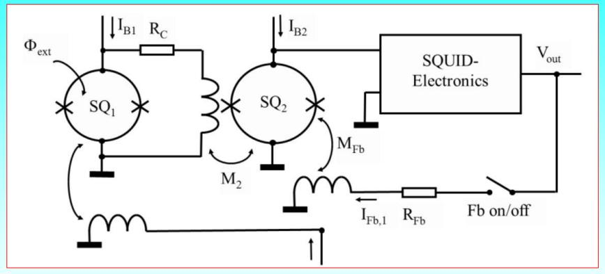
The nanoSQUID (SQ1) is voltage-biased with a parallel resistor R=1.5  $\Omega$ . The critical current change of the nanoSQUIDs is sensed with the SQUID amplifier (SQ2-parallel double-washer). Feedback from a directly coupled SQUID electronics (Supracon) is applied to the amplifier SQUID ( $S_I^{1/2}$ = 5 pA/Hz  $^{1/2}$ ).
