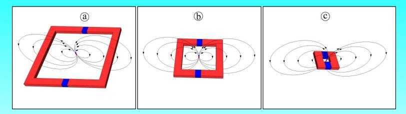
By decreasing the detection coil size, the number of flux lines which return within the loop decreases and the net magnetic flux increases.
