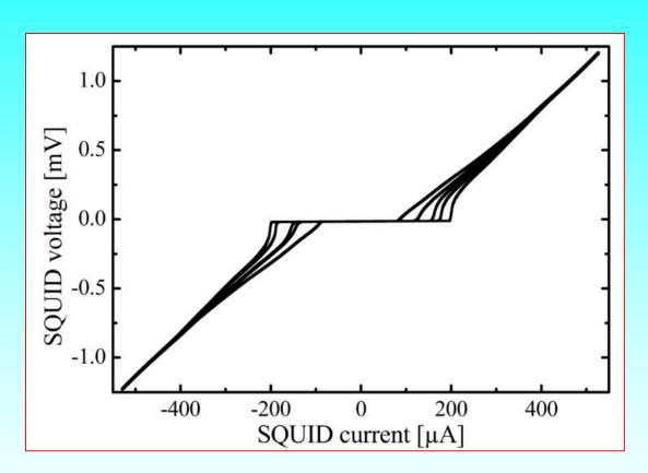
Set of current-voltage characteristics measured at 4.2 K for different magnetic flux threading the SQUID loop, ranging from 0 to 0.5  $\Phi_0$  in steps of 0.1  $\Phi_0$
