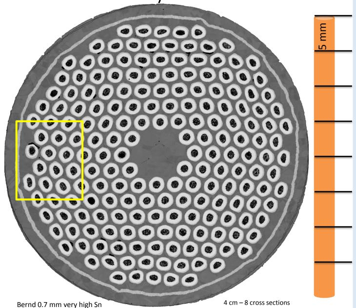
The effect of a breached filament can be much larger than suggested by a single cross-section
