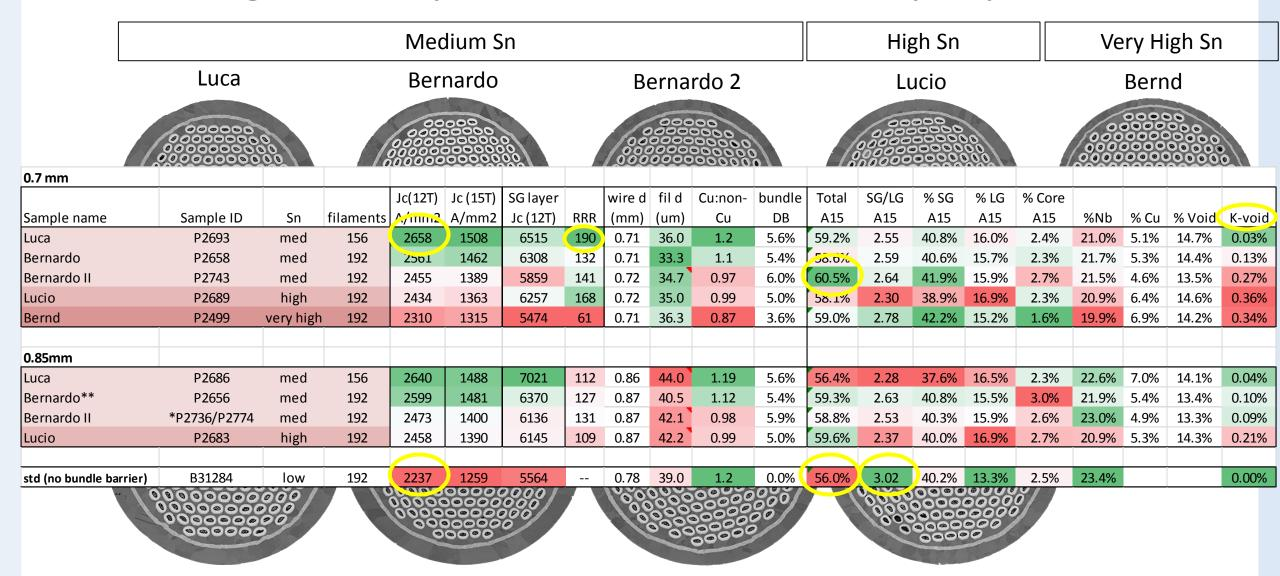
All higher J<sub>c</sub>! BUT, why doesn't J<sub>c</sub> increase with Sn content? We suspect Sn leaks
