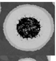
Unbreached: fully continuous barrier
