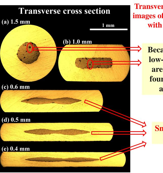
Transverse cross section optical images of superconducting tapes with different thickness
