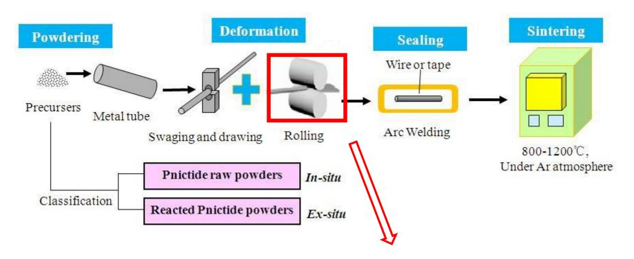
Tape thickness is an important parameter to the  $J_{\rm c}$  properties; The silver sheathed Sr-122 wires or tapes with thickness of 1.5 mm, 1.0 mm, 0.6 mm, 0.5 mm and 0.4 mm are fabricated.
