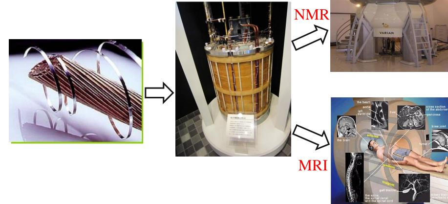
Wires and tapes are the foundation for large scale application Development of high-performance wire conductors is essential
