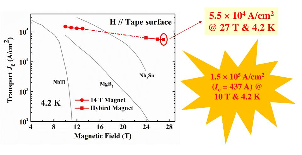
The first report of hot-pressed Ba-122 superconducting tapes; These  $J_{\rm c}$  values are by far the highest ever reported for iron-based superconducting wires and tapes
