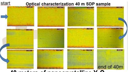
40 meters of nanocrystalline Y<sub>2</sub>O<sub>3</sub> buffer printed at 30 m/h on unpolished stainless steel
