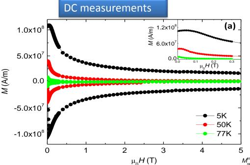
Granularity analysis  $<2a>=0.80\pm0.05~\mu m$   $J_c^G=49\pm2~MA/cm^2$  at 5K  $J_c^{GB}=15,9~MA/cm^2$  at 5K
