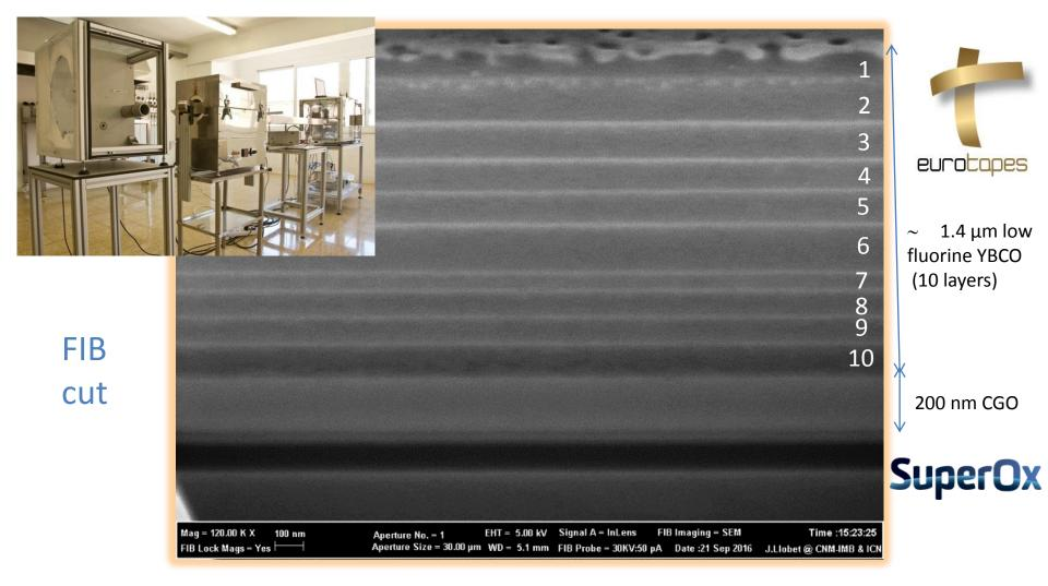
Compact layers after pyrolysis obtained by inkjet printing multi-deposition Cu-rich interlayers are visible between the multideposited YBCO films.
