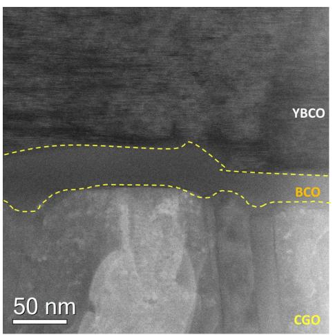
The formed BCO doesn't seem to disturb the epitaxial growth of YBCO on top; the major part from the 200 nm of CGO remains unreacted.
