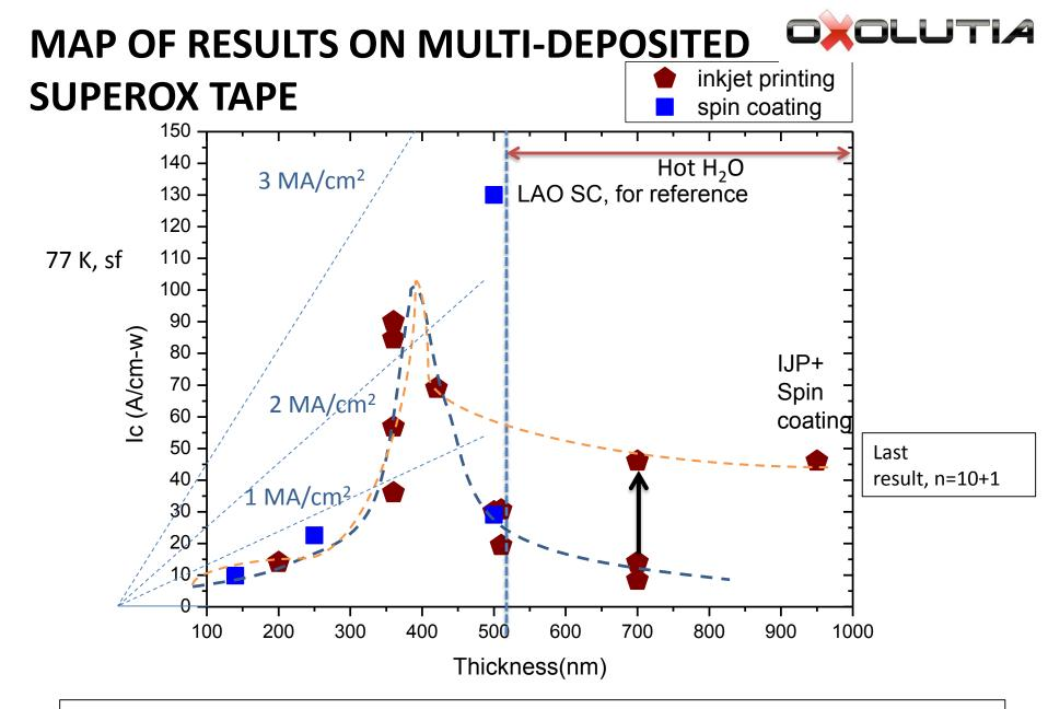
Observations: still n=5 is highest in Ic. Slower pyrolysis ramps in  $O_2$  produce flatter samples and this is main limitation for Ic enhancement. Growth conditions become more and more relevant too for top results in thicker films
