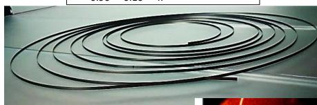
10 meters of (001)-oriented (Ce,Zr)O<sub>2</sub> buffer printed at 28 m/h
