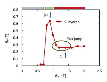
Large temperature rise causes the flux jump and flow
