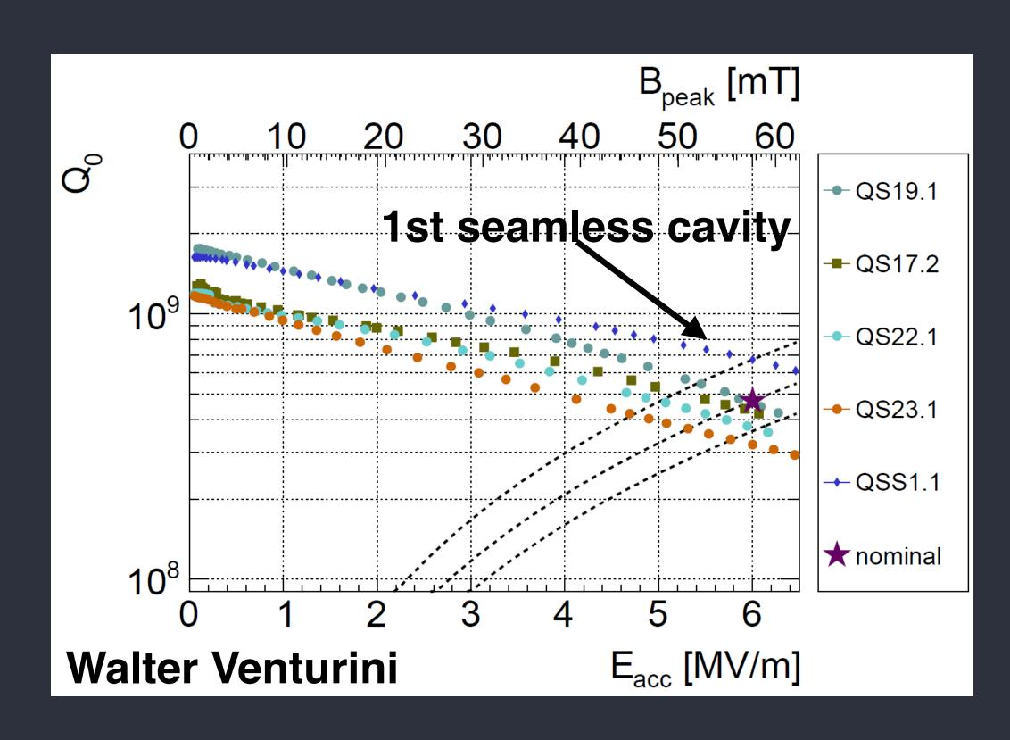
Cold test results of cavities for 4th module
