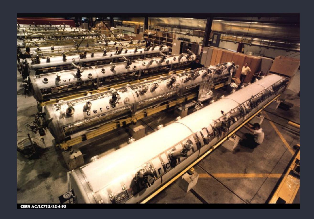
In 1999 288 SC cavities were installed in LEP
