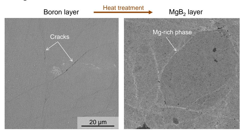
The low  $J_c$  of wire 3 is because supercurrent is blocked by Mg-rich phase, which is formed by the condensation of Mg to the cracks of the boron layer.
