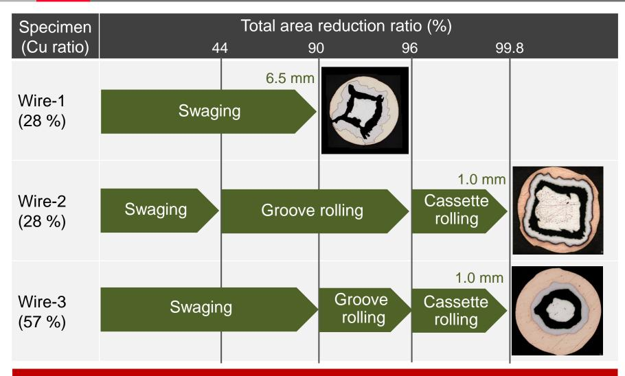
In wire-3, we thinned 1.0 mm in diameter and the length reached 100 m. Thicker Cu is effective to make the thickness of sheath homogeneous.
