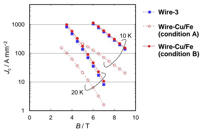
In the case of Cu-stabilized wire, it was more difficult to find a suitable condition because Cu is soft. Now, we found the condition where high  $J_c$  is obtained.
