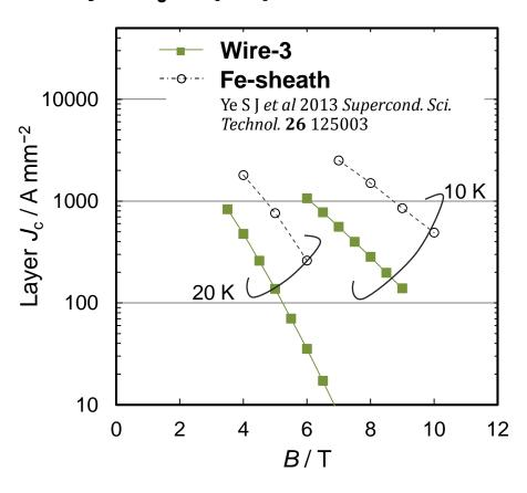
The microstructure of the  $MgB_2$  layer in Wire-3 seems to be good, but the layer  $J_c$  is not so high.
