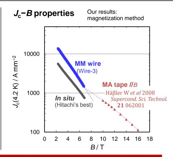
The MM wire has higher  $J_c$  than Hitachi's best in situ wire.
