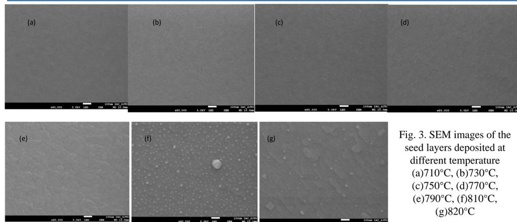
Fig. 3. SEM images of the seed layers deposited at different temperature (a)710°C, (b)730°C, (c)750°C, (d)770°C, (e)790°C, (f)810°C, (g)820°C
