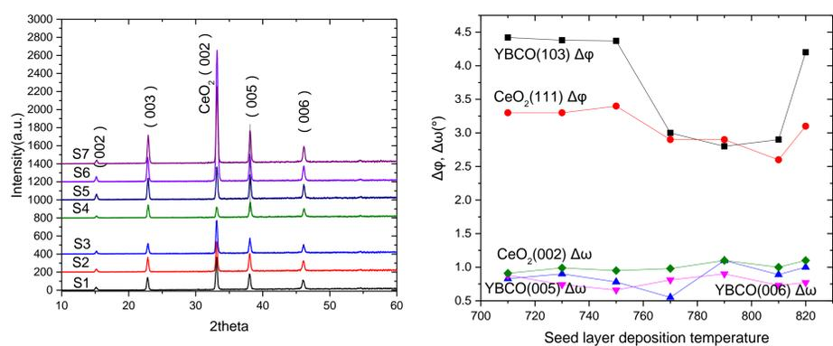
Fig. 2. (a) XRD  $\theta$ - $2\theta$  patterns of all the samples, (b) FWHM values of YBCO (103)  $\phi$  scan, CeO<sub>2</sub>(111)  $\phi$  scan, YBCO (005)  $\omega$  scan, YBCO (006)  $\omega$  scan and CeO<sub>2</sub> (002)  $\omega$  scan.
