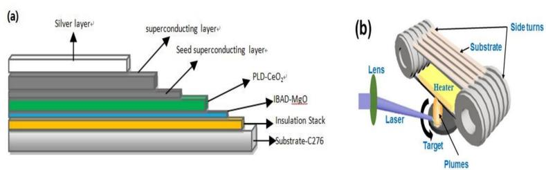
Fig. 1. Schematic diagrams of the cross section of coated conductor architecture based on IBAD-MgO templates (a) and a reel-to-reel PLD system (b).
