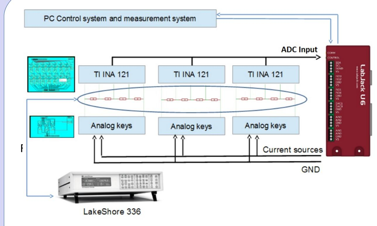
The Measurement system was based on a LabJack U6 pro ADC system and a Lakeshore 336 temperature controller.
