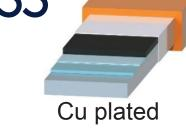
Homogenous thickness is important for high density packing of turns and reproducible coil thickness
