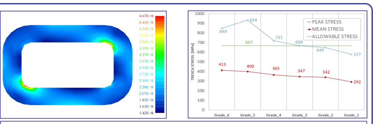
The stress peaks (used for fatigue analysis) are always located at inner Jacket fillets, with a stress value higher than the allowable one (667 MPa), except that for the first and second double layer. Mean stress values of each layer is lower than the allowable value, with a minimum safety factor of about 1,6.
