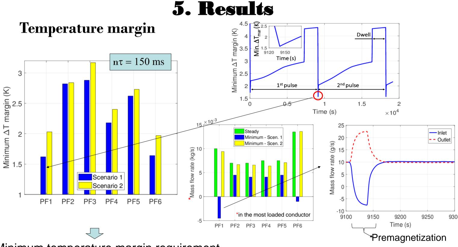
Minimum temperature margin requirement  $(\Delta T_{mar} > 1.5 \text{ K})$  is always fullfilled
