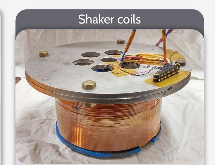
Pair of copper solenoids connected in series, used to generate the axial AC field (max. amplitude 80 mT)
