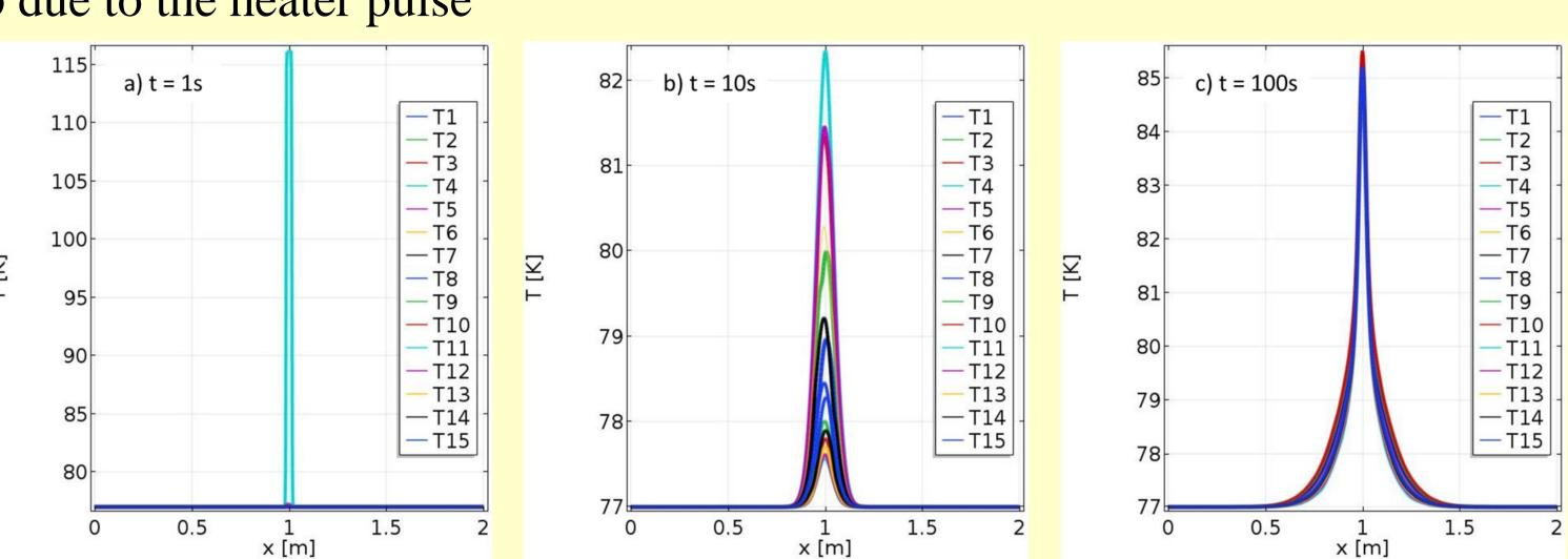
After few seconds the temperature redistributes and at  $100 \, s$  the tapes show the same temperature profile determining the quench of the cable.
