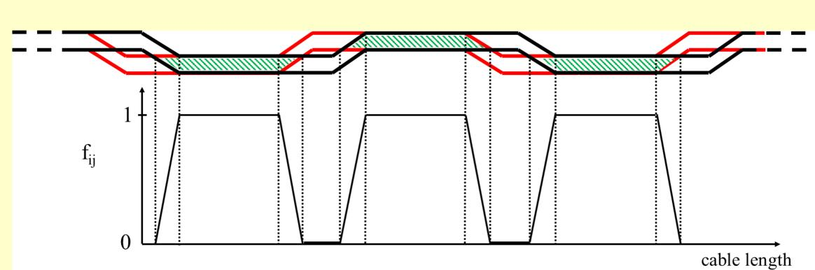
The function is equal to one if the two tapes overlap while zero if they are not in contact
