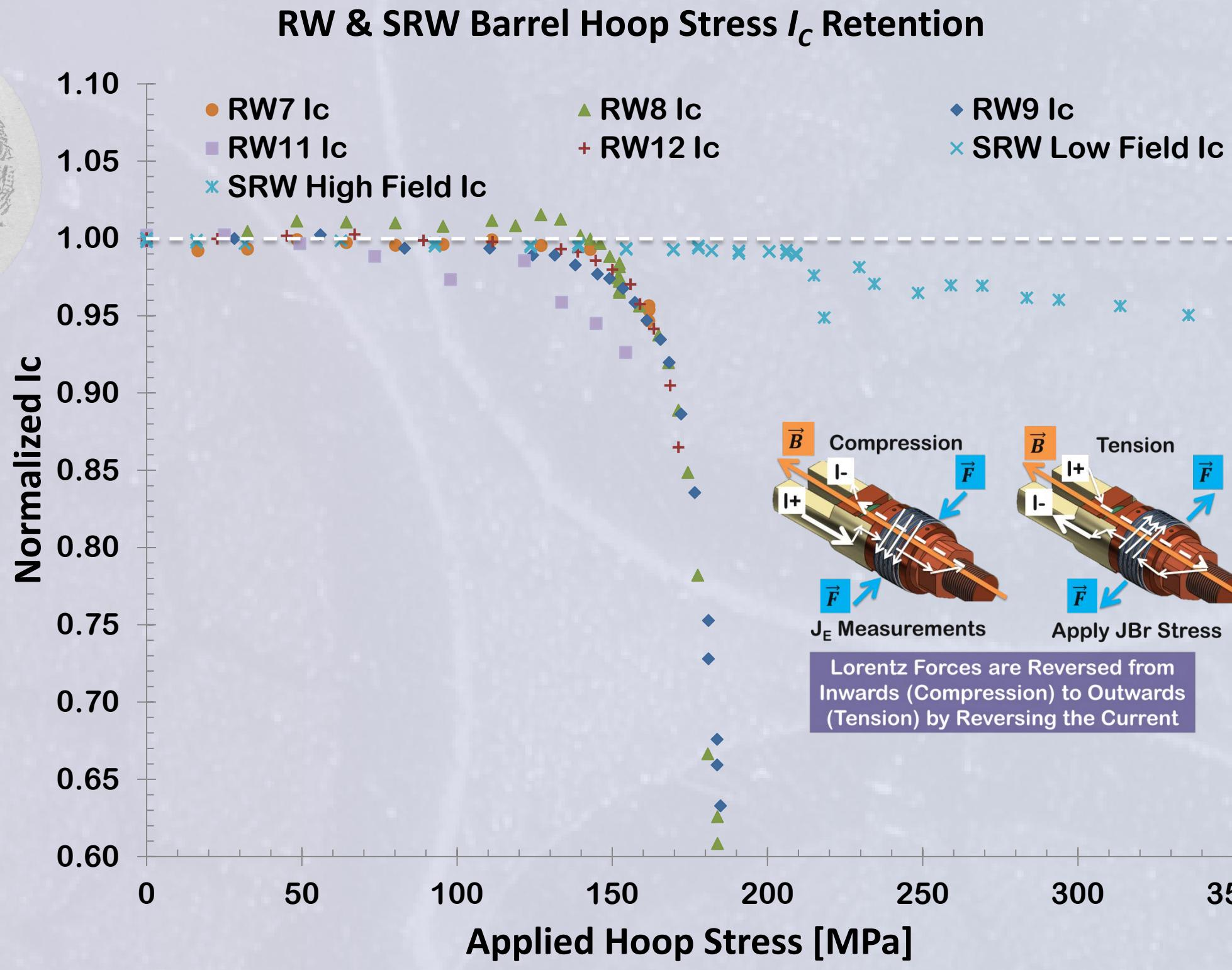
Round-Wire barrel  $I_c$  retention is independent of 2212-powder or wire architecture
