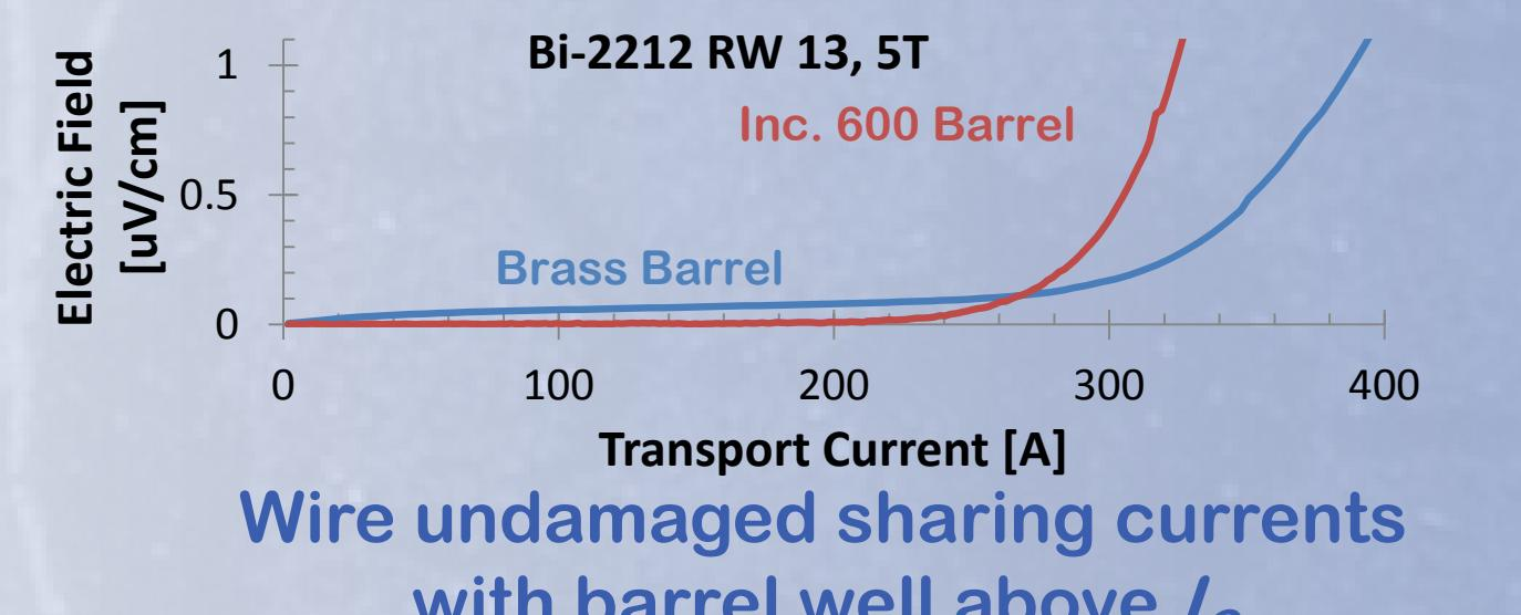
Wire undamaged sharing currents with barrel well above  $I_c$
